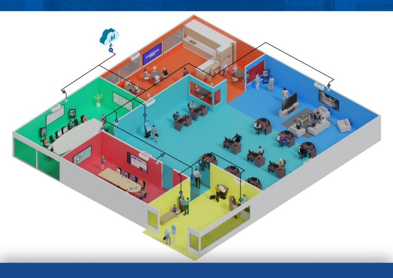
A network of smart occupancy sensors, can provide valuable data and insights to a live dashboard, or generate reports, to optimise real estate planning, room utilisation and health management through the spacing of staff. The smart sensors can be fully integrated into the EzeImpress CMS platform.
